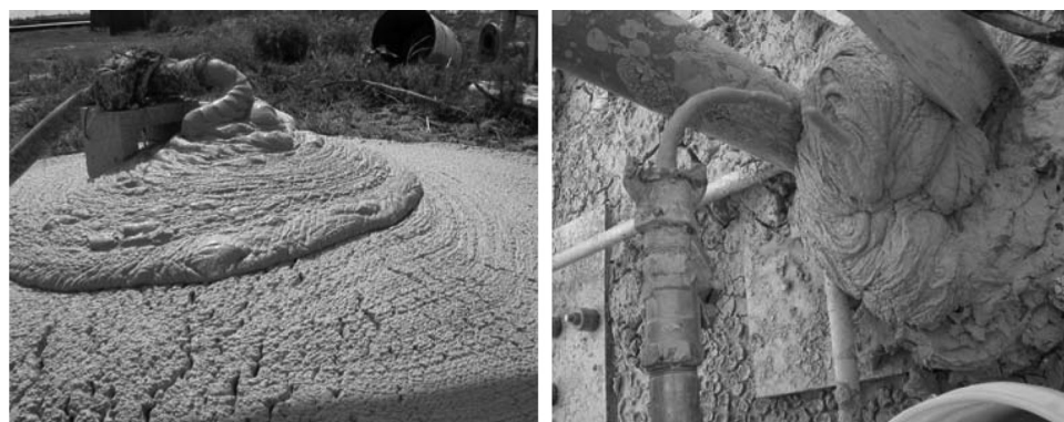
FIG. 13. Pictures of paste products with high solids.
