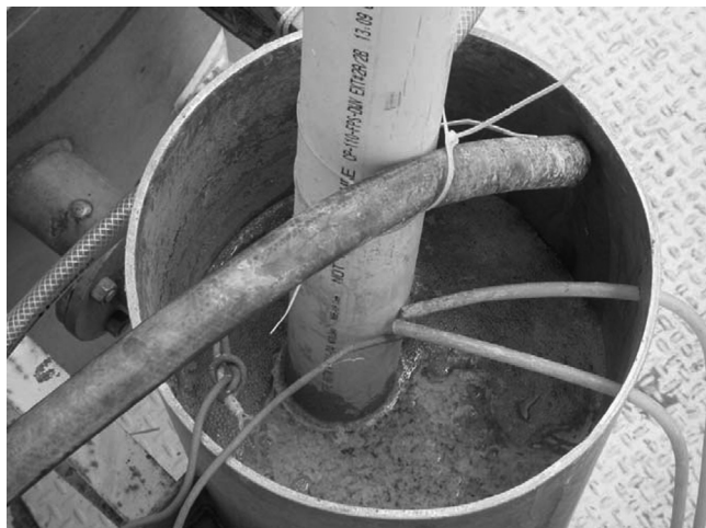
FIG. 6. Flocculation inside conditioning tank beside DCT where Hengfloc 80607 was added.
